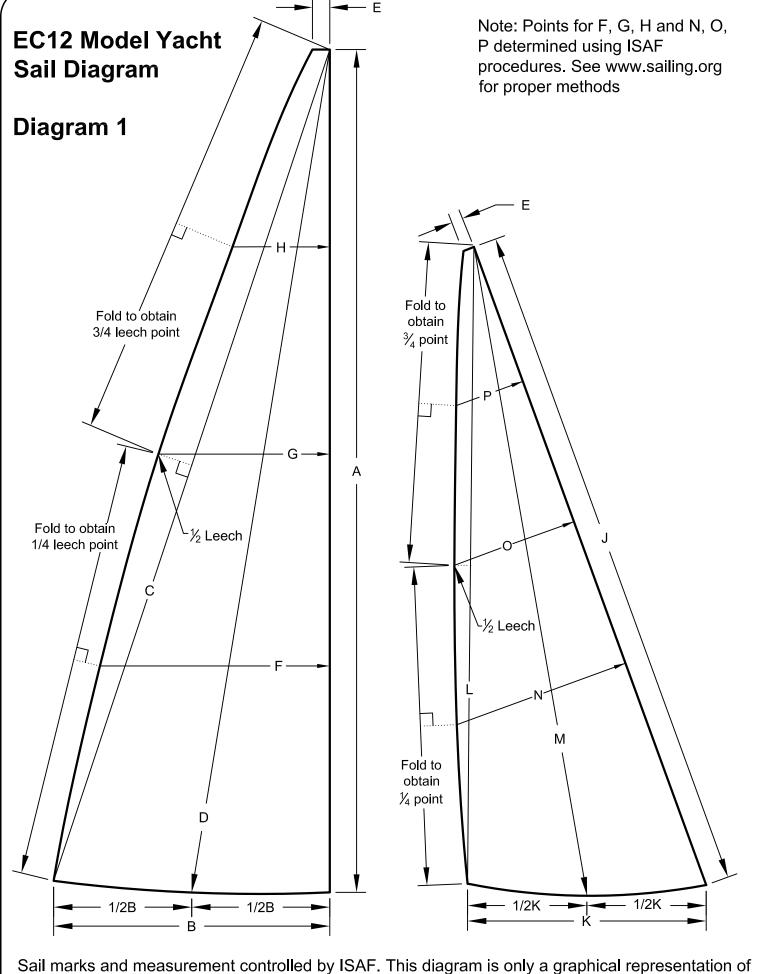
Sail marks and measurement controlled by ISAF. This diagram is only a graphical representation of ISAF Rules and procedures. For more information or measuring procedures, see www.sailing.org.
